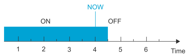
Indoor unit set to stop in 0.5 hours.
